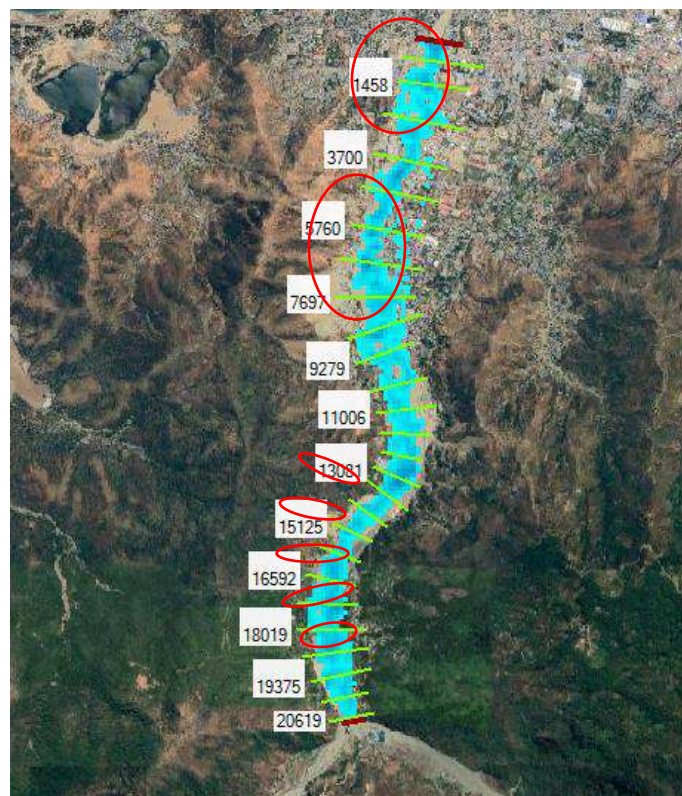
Figure 5. Location of embankment construction and normalisation
