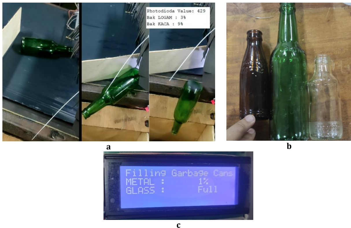
Figure 14 The result of the glass waste sorter; a. Implementation result; b. Glass waste to be sorted. c. Display
