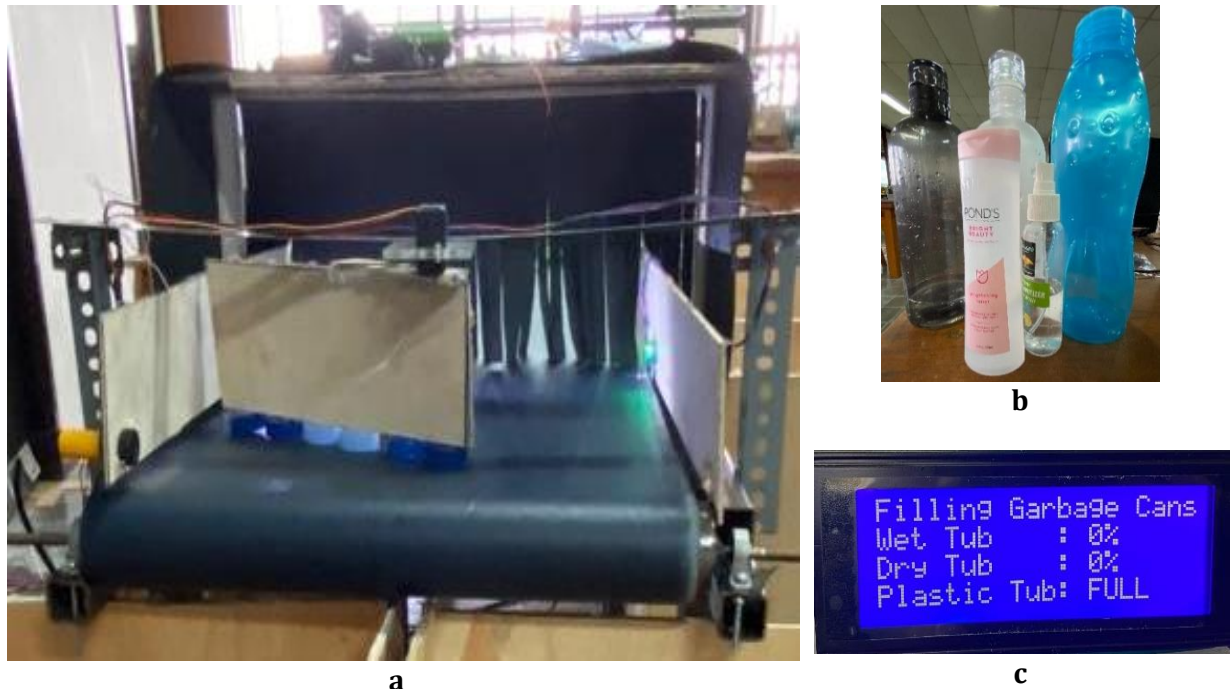
Figure 16. The result of the plastic waste sorter; a . Implementation result; b . Glass waste to be sorted; c . Display.
