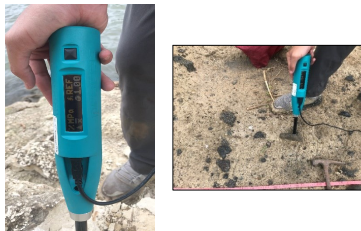
Figure 5. Example of measuring rock strength using a Schmidt hammer on calcarenite at the Sc location. 1 (left) and in andesite breccia at location Sc. 6 (right).
