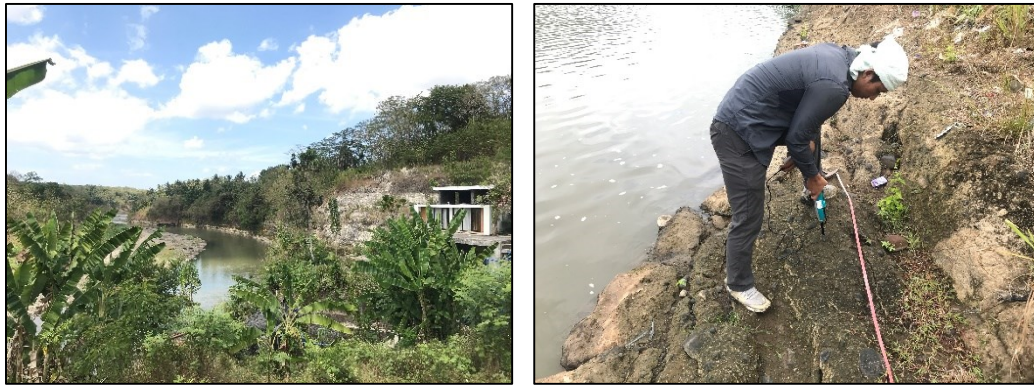
Figure 3. Slope composed of calcarenite at location Sc. 2 (left) and andesite breccia at location Sc. 6 (right).
