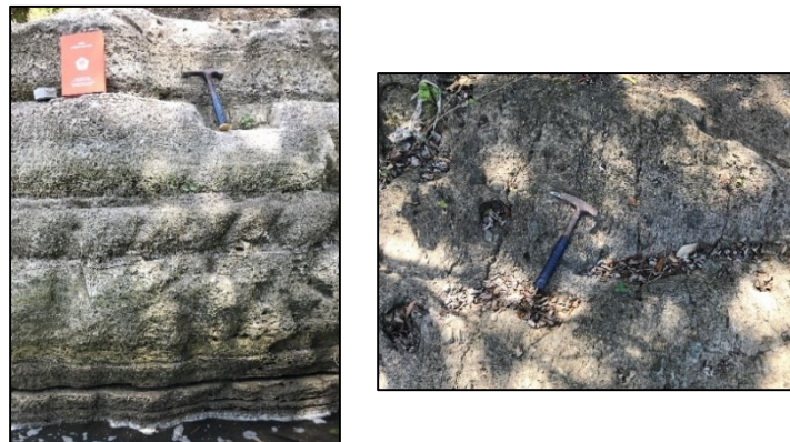
Figure 4. The discontinuity area in calcarenite (Sc. 2) is in the form of layers and joints (left), while in andesite breccia (Sc. 8) it is dominated by joints (right).
