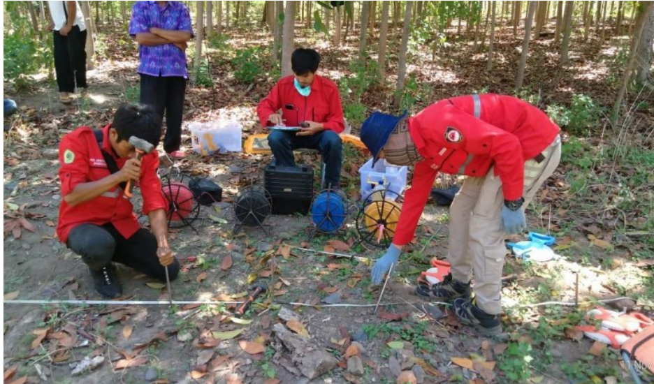
Figure 3. The process of acquiring VES Geoelectrical Resistivity data in Mumbul Sari Village, Bayan District, North Lombok.
