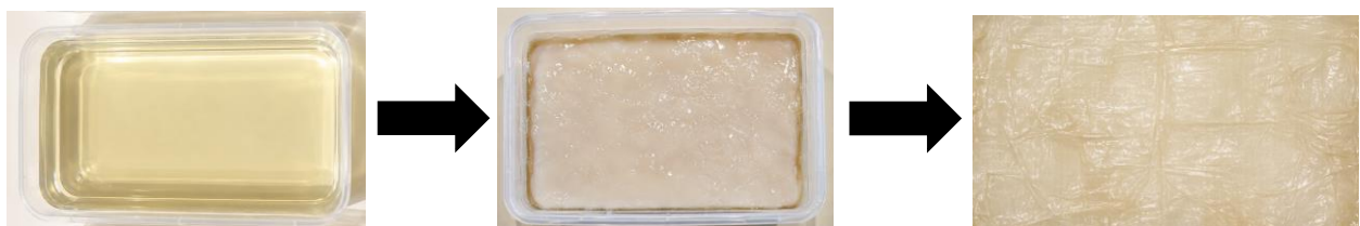
Figure 1. Transformation of anaerobic digestate into dried bacterial cellulose sheet
